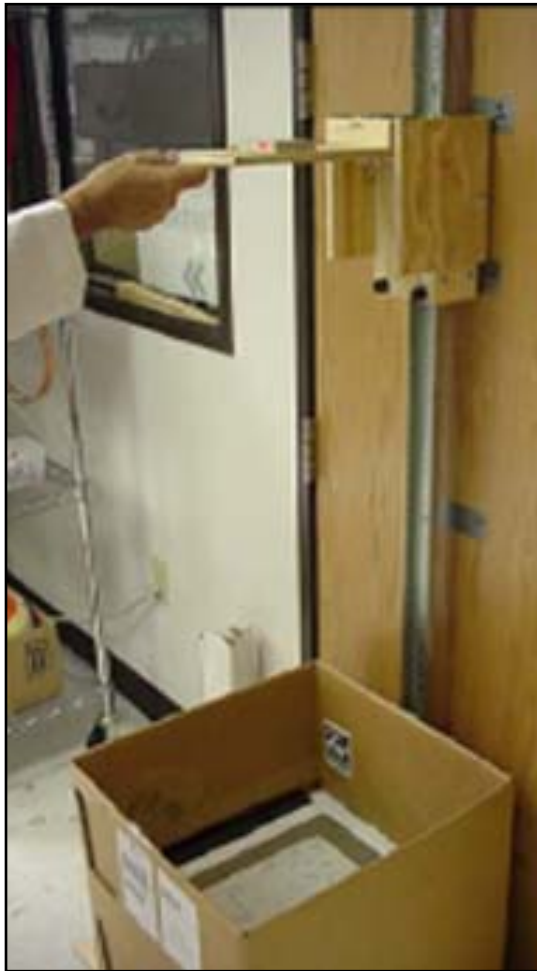
Figure 2: Drop Fixture used for Drop Testing
